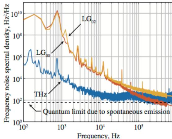
Fig.1. Frequency noise of the THz source versus dual-frequency source
