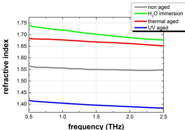
**Fig. 1.** Refractive index of different aged epoxy polymers over a frequency range 0.5 up to 2.5 THz.
