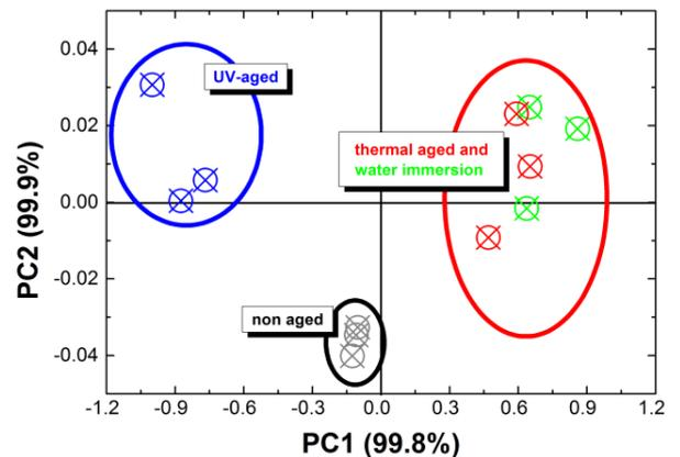
**Fig. 2.** Principle component analysis (score plot) of the refractive index spectra from different aged epoxy polymers.
