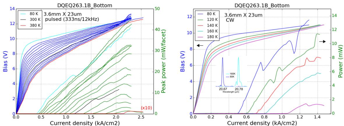
Fig.1. Electrical and optical output characteristics of InAs/AlSb QCL emitting above 20  $\mu\text{m}$  in pulsed mode regime (left), and continuous wave regime (right). Insets show emission spectra in continuous wave regime.
