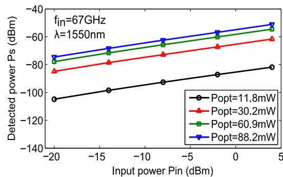
Fig.2. Detected power for an input signal at a frequency of 67 GHz for variable input power
