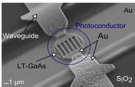
Fig.1. LT-GaAs photoconductor in resonant cavity linked to microstrip-lines
