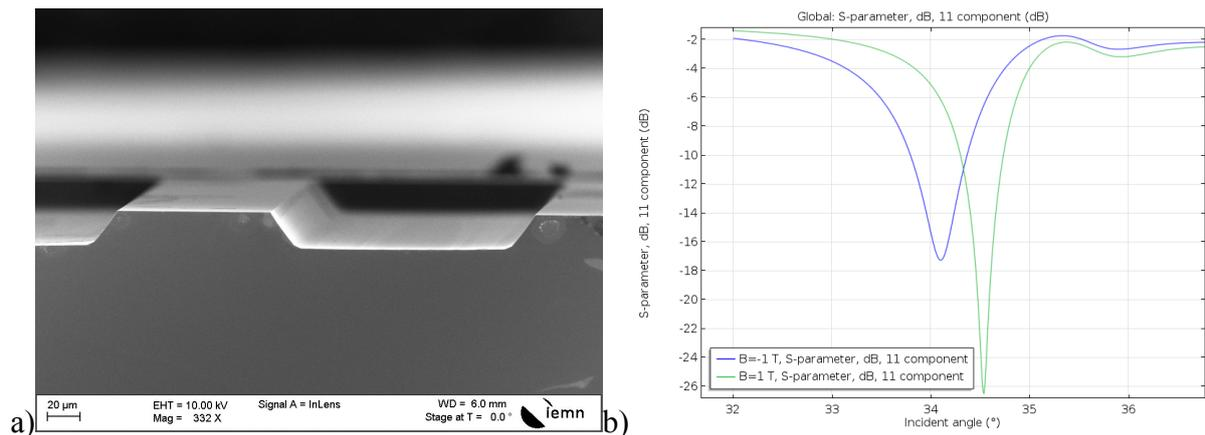
Fig.1. (a) - InAs grating with 250  $\mu\text{m}$  period and 20  $\mu\text{m}$  depth, using  $\text{H}_3\text{PO}_4:\text{H}_2\text{O}_2$  etching solution. (b) - Calculated reflectivity at 761 GHz (HCOOH THz laser line) vs incidence angle.
