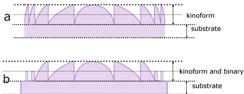
*Fig.1 Illustration of the possibility of eliminating the negative impact of shadow effect concept: a) kinoform with fast alternating phase on the edges of, b) hybrid structure consisting lens coded as kinoform in the middle and as binary structure on the edges.*
