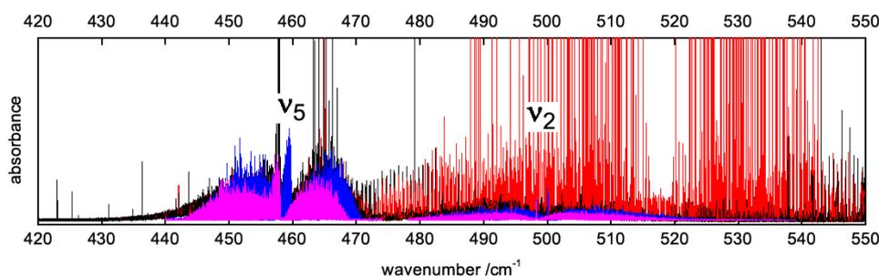
Fig. 1. Synchrotron-Based FT-FIR spectrum of  $\nu_5$  and  $\nu_2$  bands of  $\text{SOCl}_2$  mixed with a strong  $\text{SO}_2$  band (in red)
