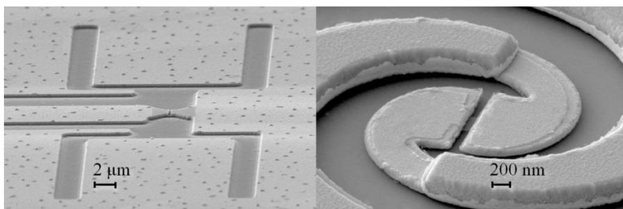
*Fig.1. (left) SEM picture of an ultra-fast YBCO detector coupled with planar antenna; (right) SEM picture of an ultra-fast NbN detector with broadband log-spiral antenna for 1 - 6 THz range.*
