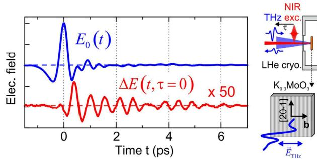
Fig. 1. An example of a pump-induced differential THz field  $\Delta E(t, \tau=0)$  for  $T=50$  K ( $h\nu_{ex}=1.6$  eV,  $F_{ex}=550 \mu Jcm^{-2}$ ) measured in reflection, with a detection bandwidth of 0.5-2.8 THz. From 2D maps of such data, we derive the transient complex conductivity  $\Delta\sigma(\omega, \tau)$  which reveals a photoinduced blue-shift of the phase-phonon bands and a dynamic broadening.
