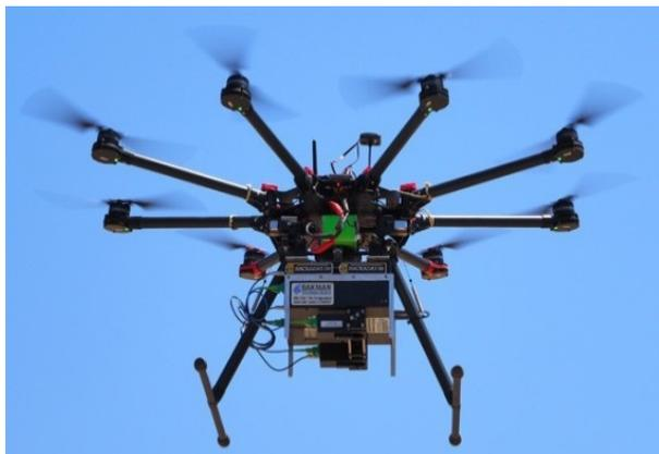
Fig.1. The modified PB7220-2000-T air-borne spectrometer attached to the drone.
