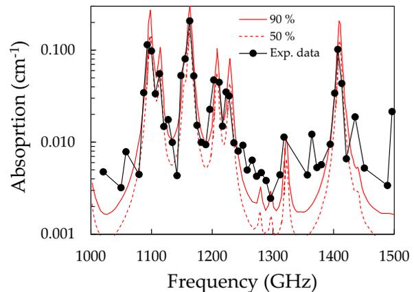
Fig.1. Recorded and calculated absorption spectra of air.
